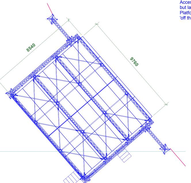
Main stage: Stage platform will be constructed of standard 'lite deck' or similar proposed dimensions 9.76m x 8.54m wide. Stage height to be set @ 0.9m DSC and levelled using screw jack system.
