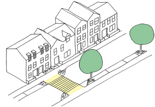
Figure 19: A sketch highlighting pedestrian crossings and on street trees - inclusion of these features can also help to reduce traffic speeds.
